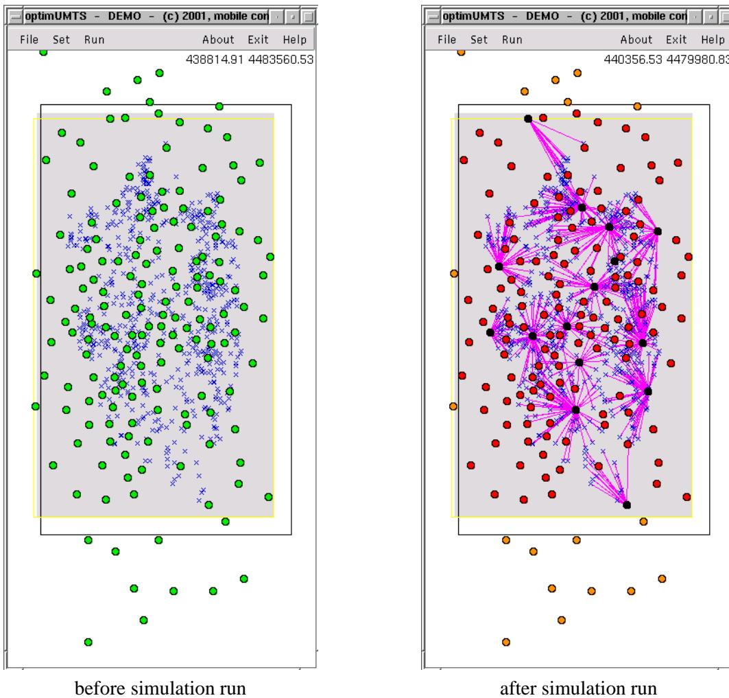
The base stations belonging to the optimized system are drawn in black, the unused base stations are drawn in red. The connection established between a mobile user and a base station is drawn with a pink line.
